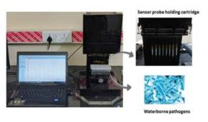
**Fiberoptic Array Biosensor:** A compact array biosensor with 8 probes for simultaneous detection of up to 7 different pathogens of interest.
