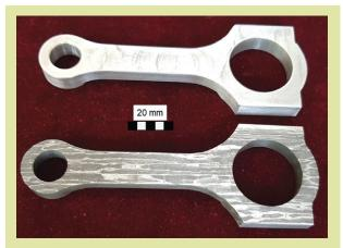
Connecting rods manufactured in igstc project nearnetmac; pure a356 al-alloy (upper part); t700 carbon fibre reinforced a356 al-alloy (lower part)
