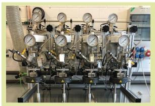
4-fold -high pressure reactor setup with feeding high pressure gas burettes at RUB for high throughput quick testing of catalysts and for kinetic measurements.
