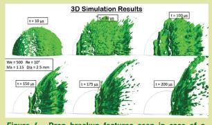
Figure 4. Drop breakup features seen in case of a 3D simulation for a high value of Weber
