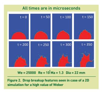
For higher Weber number, K-H instabilities are initiated near the pole on the windward side which travel towards the equator and form ligaments. The rupture of these ligaments due to the high shear gives rise to the ultimate shear-induced breakup of the drop at the high value of Weber number.
