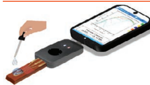
Schematic for the operation of the sensor chip integrated with smartphone
