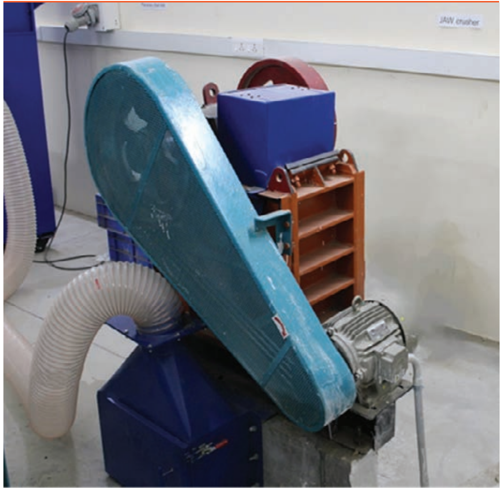
Jaw Crusher for recycled aggregate processing at IIT Madras
