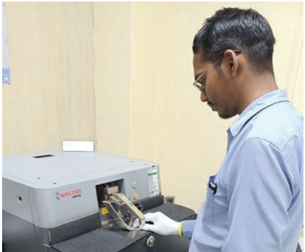
Lab spectrometer at CMR lab for spark-discharge optical emission spectroscopy (SD-OES)
