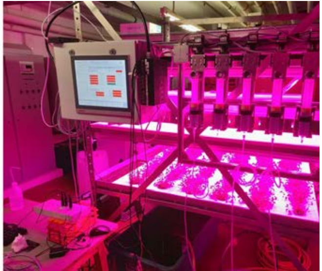
Experimental set up in the hydroponic test unit for vertical farming at Hochschule Weihenstephan-Triesdorf
