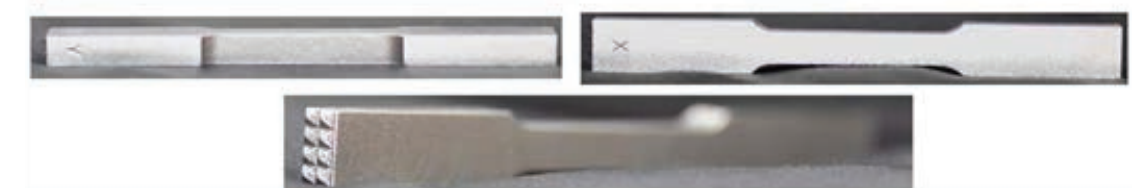
3D Printed Dog specimen from metal power
