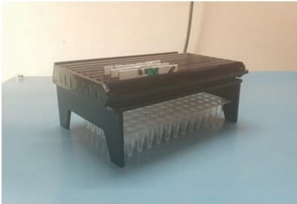
U bend probes with paper cartridge placed on the cartridge holder compatible with 96 well plates to functionalize
