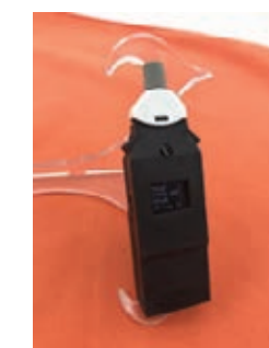
Revised prototype with integrated sensors and smaller housing
