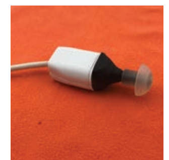
Assembled probe with injection moulded parts design-I
