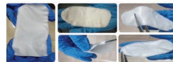
Polymer sheet dimensions (length x width x thickness): 10 cm x 6 cm x 100 μm
