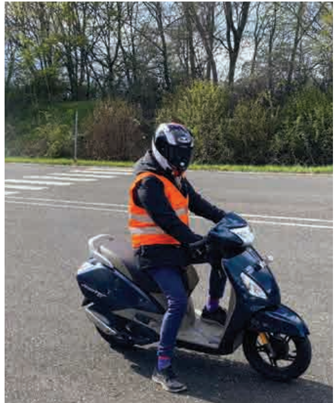
TVS Jupiter on test track gathering measurements for the vehicle model validation in Germany
