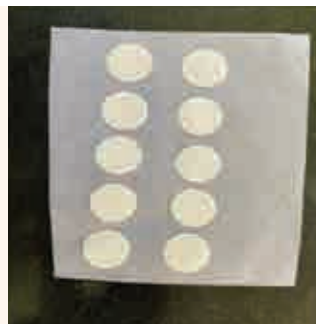
Photograph of solid electrolyte discs (2cm 2 ) obtained from the free standing film
