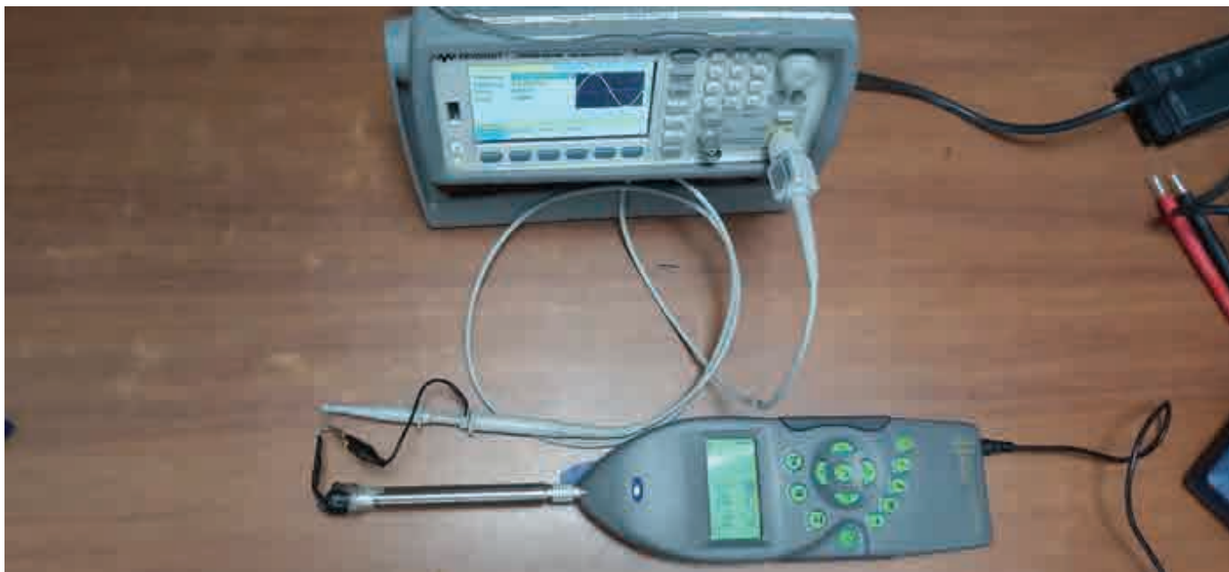
Actual experimental setup to calibrate speaker 1 and 2
