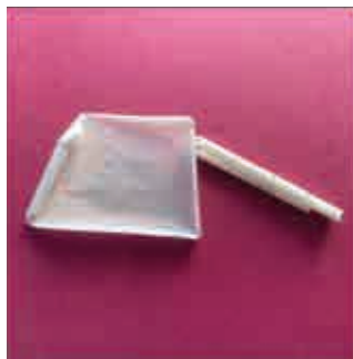
Photograph of Free standing LLZO Membrane
