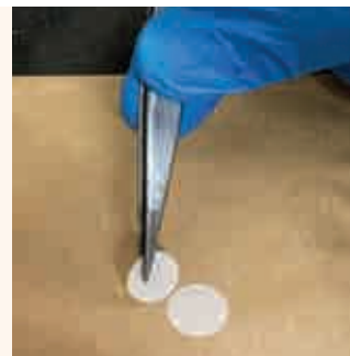
Photograph of solid electrolyte discs (2cm 2 ) obtained from the free standing film
