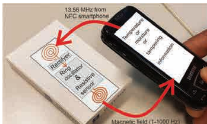
A LABELONIK label on a package communicating with a smartphone.
