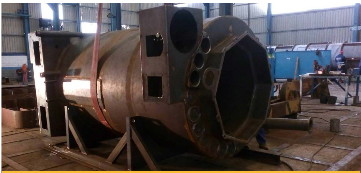
C63-F Pyrolysis machine (view on completed housing steel works).
