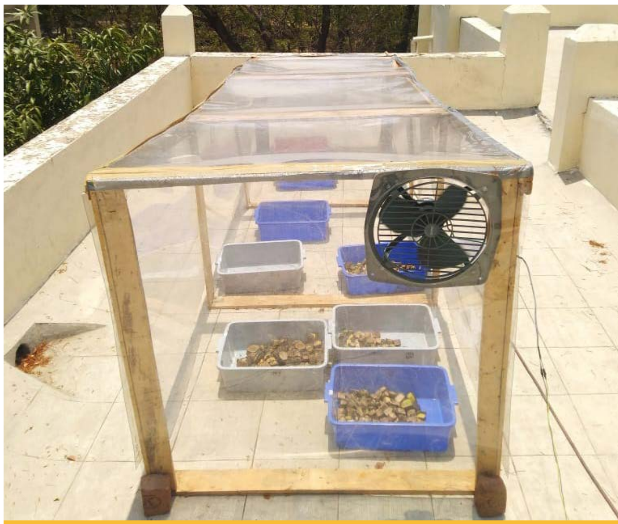
Lab scale solar dryer is set up with structure, transparent covering and drying tray.
