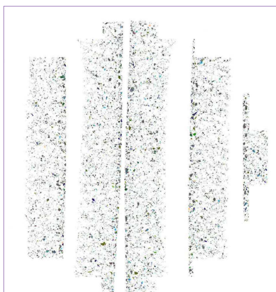
Mineral Liberation Analyzer (MLA) mapping of ore sample embedded in epoxy resin
