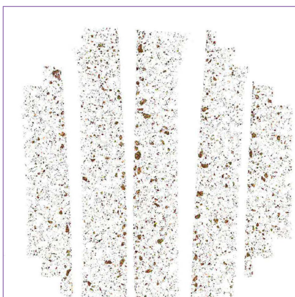
Mineral Liberation Analyzer (MLA) mapping of ore sample embedded in epoxy resin
