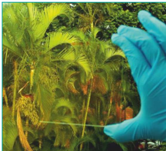
10×10 cm 2 Al mesh TCE prepared by spray pyrolysis
