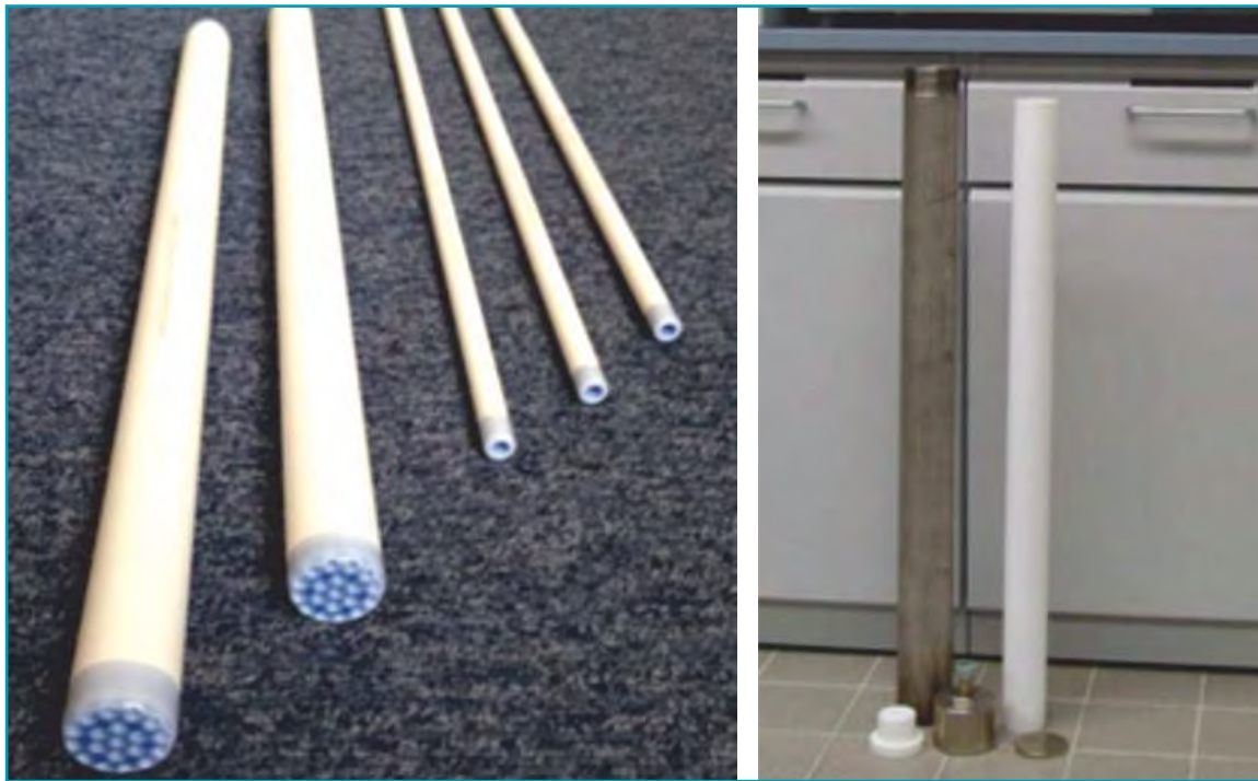
Fig. 1: Ceramic supports of 0.5 m length in single, 7 and 19 channel geometry developed by Atech (left) and 800 mm long autoclave for MFI-membrane synthesis (right)
