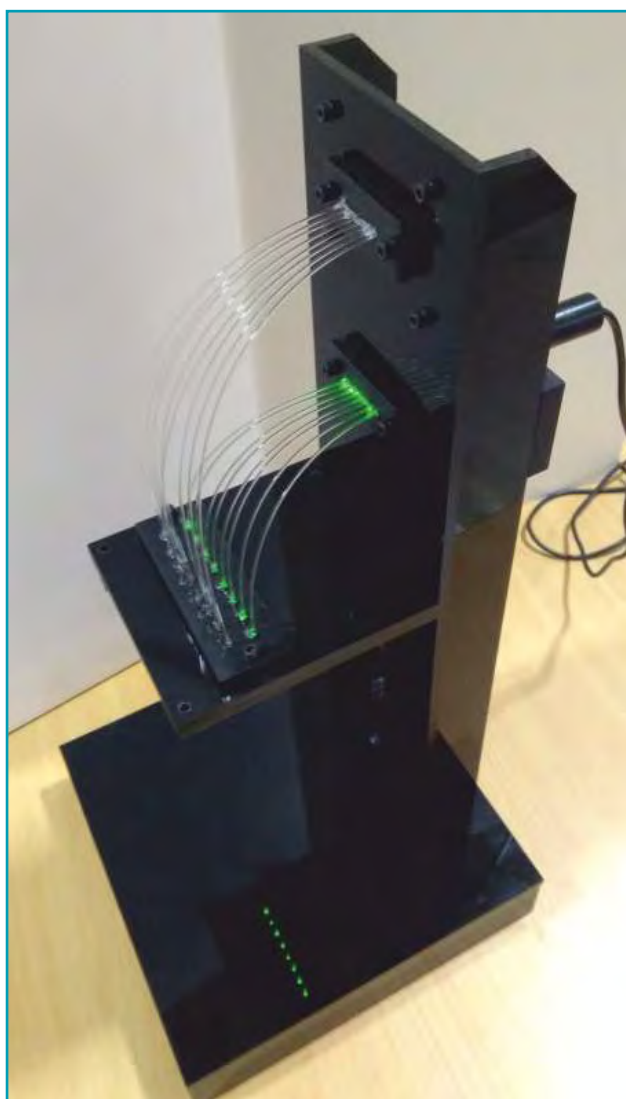
Fiber Array Sensor with Laser and CCD detector
