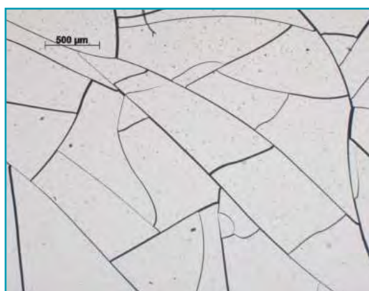
Fig. 2: Optical microscope image of the Ag-mesh network prepared on a 23 µm thick PET foil at UBT.
