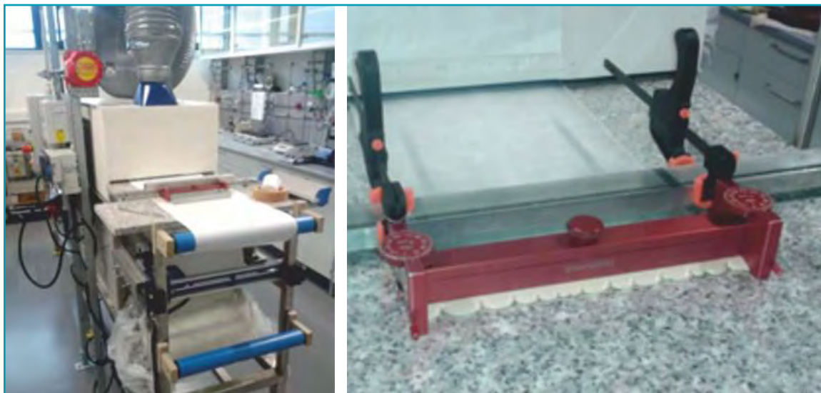
Fig. 2: Front side of the tape-casting machine (left) and knife during casting the transparent support tape with a PDMS/MFI-mixture (right)
