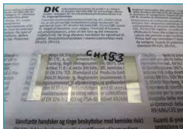
Fig. 3: Photograph of a PET foil with the Ag-mesh network prepared at UBT. The opaque metal part on the foil was used to measure the sheet resistance. The light transmission through the PET foil was 95% in the wavelength range between 300 nm and 1000 nm. The sheet resistance of the foil was 32 ohm/square.
